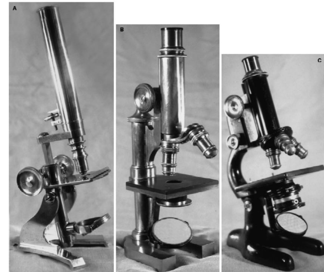
FIG. 5. (A) English brass microscope. Monocular compound microscope attributed to M. Phelps of London, England, circa 1860. (B) German brass microscope. Monocular compound microscope manufactured by E. Leitz of Wetzlar, Germany, circa 1900. (C) American microscope. Monocular compound microscope, manufactured by Bausch and Lomb, of Rochester, New York, circa 1915.
